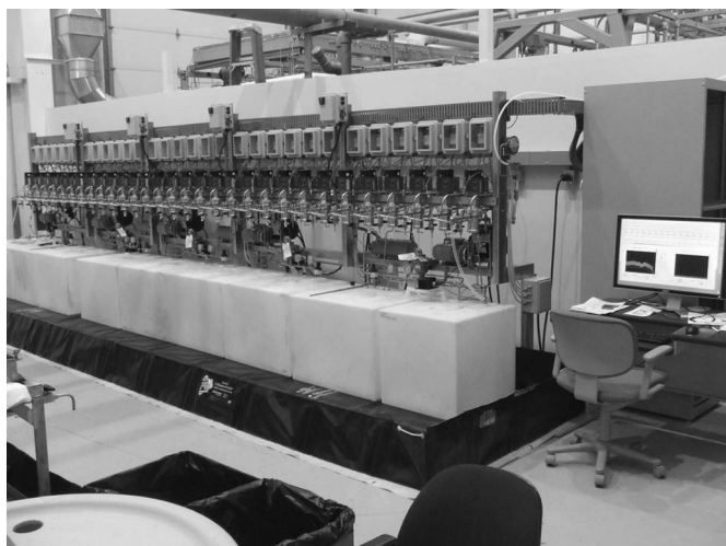
FIG. 1. Thirty stage V-02 annular centrifugal contactor pilot plant.
